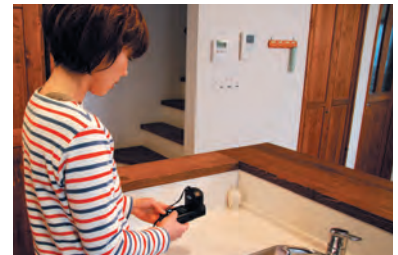
遊離残留塩素の測定 Measurement of free residual chlorine
